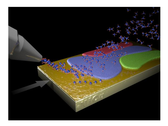
In a controlled environment, the fastest-growing orientation of graphene crystals overwhelms the others and gets "evolutionarily selected" into a single crystal, even on a polycrystalline substrate, without having to match the substrate's orientation. An Oak Ridge National Laboratory-led team developed the novel method that produces large, monolayer single-crystal-like graphene films more than a foot long. Credit: Andy Sproles/Oak Ridge National Laboratory, US Dept.
