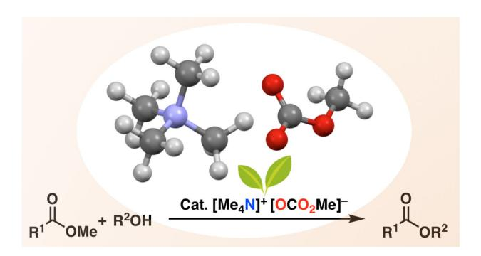
Tetramethylammonium methyl carbonate (TMC) reacts in-situ with an alcohol to form an alkoxide ion, which then attacks the starting ester to give the complex target ester in high yields. Credit: Manabu Hatano & Kazuaki Ishihara
