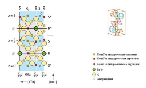
Crystal structure of M-type hexagonal ferrite (a type of magnetoplumbite). Credit: South Ural State University (SUSU)
