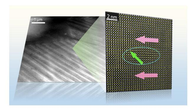
A long-range ferroelectric domain with nanoscale structure heterogeneity (4-8 nm) is evidenced by high-resolution TEM. Credit: Fei Li/Penn State
