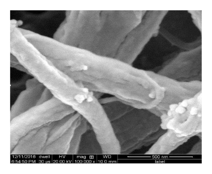
Specks of titanium dioxide adhere to polyvinyl fibers in a mat developed at the Rice University-led NEWT Center to capture and destroy pollutants from wastewater or drinking water. After the mat attracts and binds pollutants, the titanium dioxide photocatalyst releases reactive oxygen species that destroy them. Credit: Rice University/NEWT
