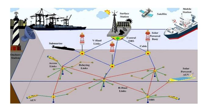
KAUST researchers are modeling various techniques for improving wireless underwater sensor networks. For example, new wireless hybrid sensors that use both acoustic and optical communication could improve underwater data collection for ocean observation. Credit: © 2018 Abdulkadir Celik
