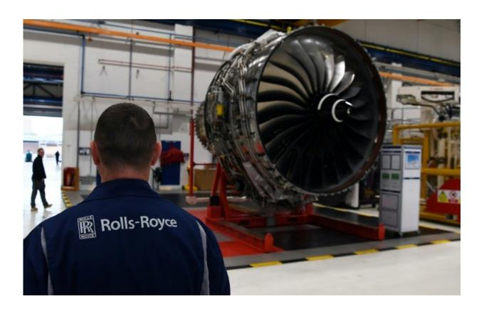
A Rolls-Royce Trent XWB aircraft engine on the assembly line at the firm's factory in Derby, England.
