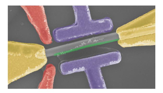
Device that physicists used to spot the clearest signal yet of Majorana particles. The gray wire in the middle is the nanowire, and the green area is a strip of superconducting aluminum. Credit: Hao Zhang/QuTech
