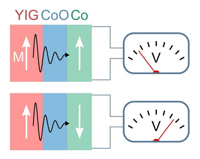
Depending on the magnetic configuration of the spin valve, the electrical signal is transmitted (bottom) or suppressed (top). Credit: Joel Cramer
