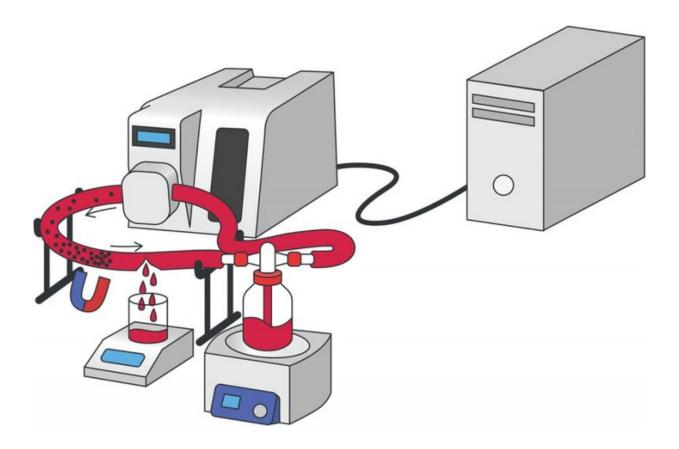
A system simulating the conditions of a damaged blood vessel. Credit: E. M. Shabanova, Andrey S. Drozdov et al.
