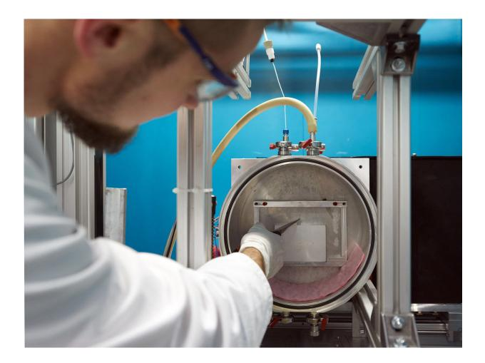
The fact that neutrons are hardly absorbed by the metal housing makes them ideal for battery research. Utilizing the neutron imaging and tomography facility ANTARES of the research neutron source FRM II, developers from Bosch and scientists at the Technical University of Munich (TUM) now used neutrons to analyze the filling process of lithium ion batteries with electrolytes. Credit: Wenzel Schuermann / TUM
