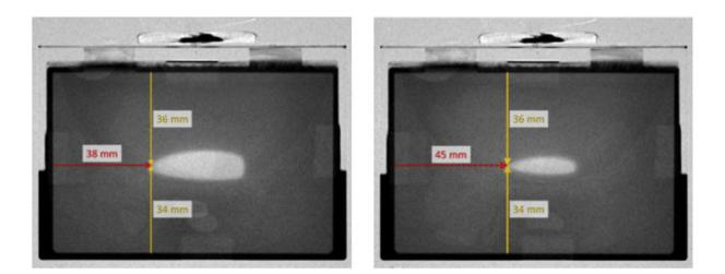
Battery manufacturers often wait several hours to ensure the liquid is fully absorbed into the pores of the electrode stack. In the light of the neutron beam scientists at the Technical University of Munich saw that in a vacuum the electrodes were wetted completely in just over 50 minutes. The image shows the wetting progress after 33 and 41 minutes. Credit: Wolfgang Weydanz / Bosch / TUM
