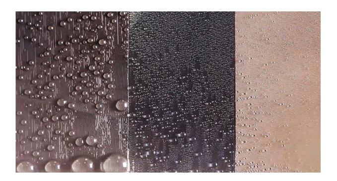
Directional slippery rough surface outperforms slippery liquid-infused porous surface (SLIPS) and conventional superhydrophobic surfaces in water harvesting in air. Credit: Xianming Dai, Jing Wang, and Tak-Sing Wong
