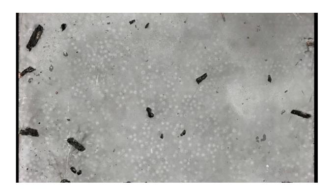
This image shows the CMF panel after the test. The black marks are fragments trapped inside the panel. The image shows there are no cracks or physical bowing -- even after the frags struck at speeds of 5000 feet per second. Credit: North Carolina State University
