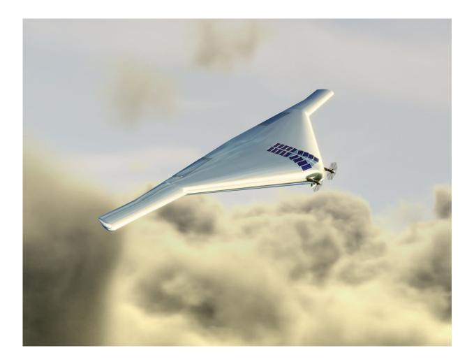
A Venus Atmospheric Maneuverable Platform, or VAMP. The aircraft, which would fly like a plane and float like a blimp, could help explore the atmosphere of Venus, which has temperature and pressure conditions that do not preclude the possibility of microbial life. Credit: Northrop Grumman
