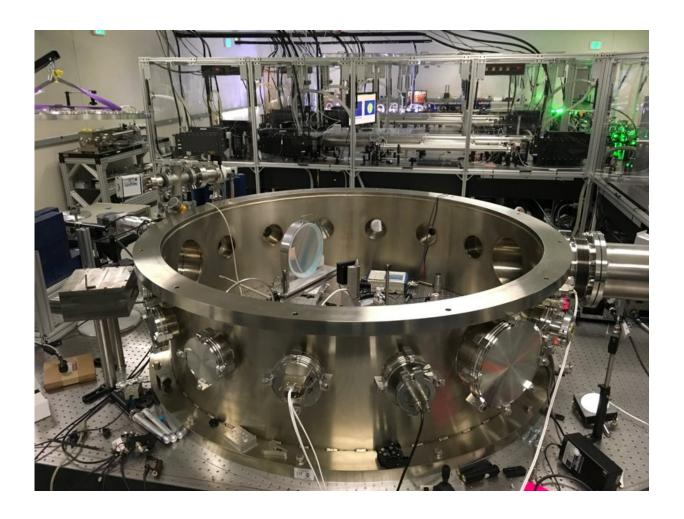
The target chamber (front) and ultra-high intensity laser (back) used in the microscale fusion experiment at Colorado State University. Credit: Advanced Beam Laboratory/Colorado State University
