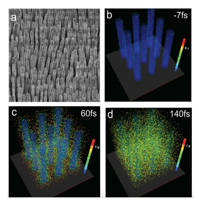
Top left: A scanning electron microscope image of aligned deuterated polyethylene nanowires. The other panels are 3-D simulations of the nanowires rapidly exploding following irradiation by an ultra-intense laser pulse. Credit: Advanced Beam Laboratory/Colorado State University
