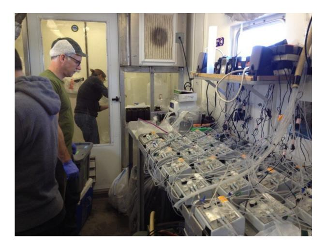
Lead author Jeff McQuaid watches an array of pumps designed to test the effects of high CO<sub>2</sub> on Ross Sea phytoplankton in Antarctica. Several recent studies have noted that high CO<sub>2</sub> has a negative effect on phytoplankton growing in low iron environments like the Southern Ocean Credit: A.E. Allen
