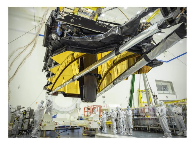
The combined optical element and science instruments of NASA's James Webb Space Telescope were removed from their specially designed shipping container, called the Space Telescope Transporter for Air, Road and Sea (STTARS), in a high bay at Northrop Grumman in Redondo Beach, California, on March 8, 2018. Credit: NASA/Chris Gunn
