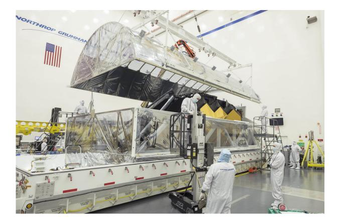
Engineers open the interior tent frame of the Space Telescope Transporter for Air, Road and Sea (STTARS) at Northrop Grumman in Redondo Beach, California, on March 8, 2018, to reveal its precious cargo -- the combined optics and science instruments of NASA's James Webb Space Telescope. Credit: NASA/Chris Gunn
