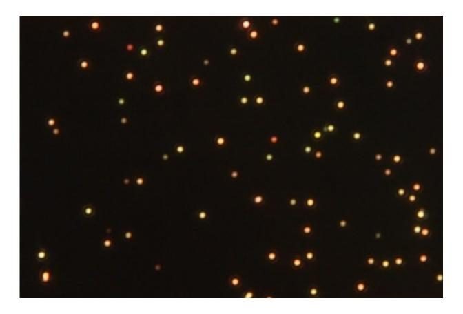
Under a standard microscope, these plasmonic nanoparticles may seem identical, but an image captured by a snapshot hyperspectral imaging system developed at Rice University shows just how different they are. The system images multiple nanoparticles and their plasmonic responses – the light they emit when excited – to show how they differ due to defects or differences in their size or shape. Credit: Rice University
