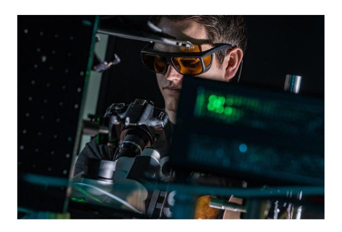
Rice University graduate student Kyle Smith checks a sample while testing the lab's snapshot hyperspectral imaging system. Rice scientists developed the system to take instantaneous spectra of multiple plasmonic nanoparticles. Credit: Jeff Fitlow
