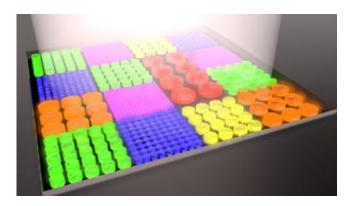
Cylindrical silicon nanoparticles of different sizes reflect light across a wide gamut of colors. Credit: A\*STAR Data Storage Institute
