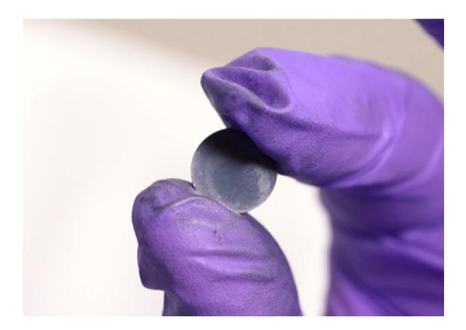
A graphite pellet made by hand from crushed graphene powder. The strong, light pellets developed at Rice University hold promise for electronic and catalytic applications. Credit: Rice University
