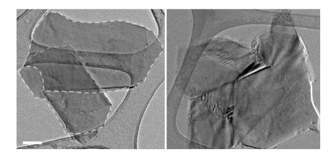
Scanning electron microscope images show graphene flakes before compression, at left, with individual flakes outlined, and well-connected graphene sheets after compression at right. Scale bar is 20 nanometers. Credit: Ajayan Research Group/Rice University
