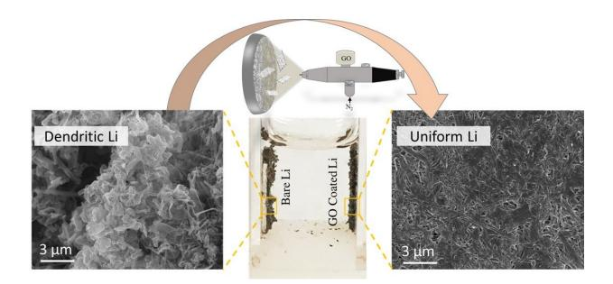
Left: Dendrites forming on a lithium electrode. Right: Lithium plates uniformly on a lithium electrode in a battery with a graphene oxide nanosheet separator. Credit: Reza Shahbazian-Yassar.
