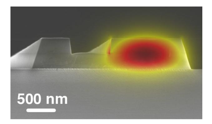
The scanning electron micrograph of a fabricated photonic waveguide used in onchip mid-infrared frequency comb lasers. Credit: National Institute of Standards and Technology, Applied Physics Division, Quantum Nanophotonics group
