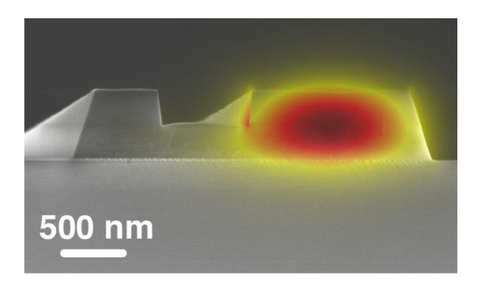
The scanning electron micrograph of a fabricated photonic waveguide used in onchip mid-infrared frequency comb lasers. Credit: National Institute of Standards and Technology, Applied Physics Division, Quantum Nanophotonics group
