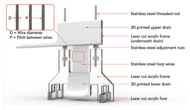
To test the fog harp's design, researchers constructed small-scale models of vertical wire arrays that could be placed inside an environmental chamber with artificial fog. The team discovered that water collection efficiency continued to increase with smaller and smaller wires.
