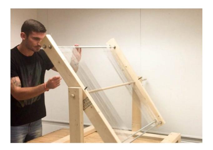
Study co-author Josh Tulkoff constructs a large prototype of the fog harp, which consists of a vertical array of 700 wires and is based on initial experimental results. Tulkoff was part of an interdisciplinary research team at Virginia Tech that discovered parallel wire arrays could increase the water collection capacity of fog nets by threefold. Credit: Virginia Tech
