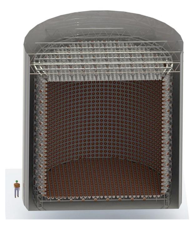
A cutaway view of the Watchman antineutrino detector The outer stainless steel tank will be approximately 16 meters tall and 16 meters in diameter and will contain some 3,500 metric tons of water. An inner structure of trusses and cables will support about 3,000 photomultiplier tubes: powerful light sensing devices that convert Cherenkov light arising from the antineutrino interactions in the
