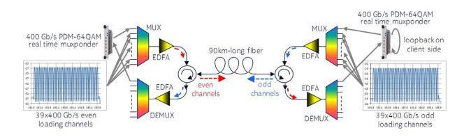
A bi-directional transmission set up with the same 90-kilometer fiber, where the even and odd 400 Gb/s channels, with the same 50 GHz grid spacing, transmit in opposite directions. Credit: Nokia
