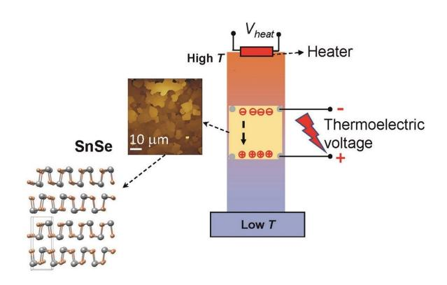
Electric charges in a nanostructured tin selenide (SnSe) thin film flow from the hot end to the cold end of the material and generate a voltage. Credit: Xuan Gao
