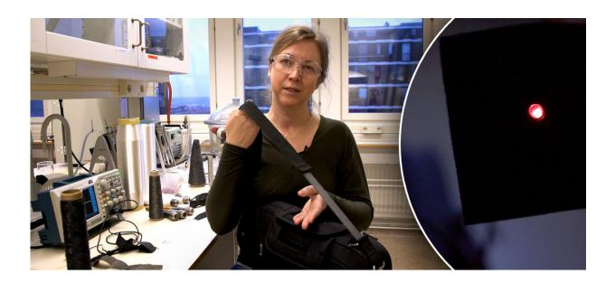
Anja Lund with a piece of the electric textile in the shoulder strap of a bag (the lighter-coloured part). To the right: a LED that flashes because electricity is generated when the textile is stretched. Credit: Johan Bodell/Chalmers University of Technology
