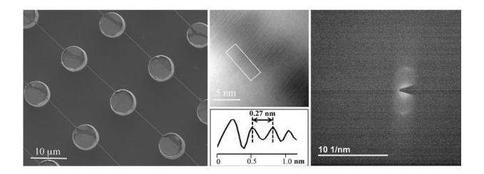
From left to right: SEM image of DNA bundles homogeneously suspended over a superhydrophobic device. In the related HRTEM image the fringes have a spacing of 2.7 Å, in good agreement with the diffraction pattern: both cases show the distance between two bases in the DNA double helix. Credit: Monica Marini
