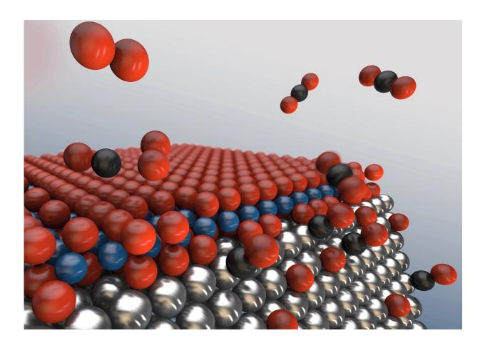
With increasing oxygen (red) concentration, an oxide sandwich forms on the surface of the metallic nanoparticles, inhibiting the desired reaction of carbon monoxide to carbon dioxide. At the edges, however, the oxide sandwich brakes up, leaving free active sites for catalysis. The more edges the nanoparticles posses, the more efficient will the catalytic converter work. Credit: DESY, Lucid Berlin
