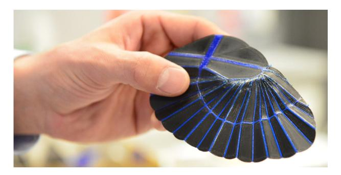
The 3-D-printed imitation of the earwig wing can be folded as compact as its natural counterpart. However, the automatic folding function so far only works in the simplified prototypes. Credit: ETH Zurich
