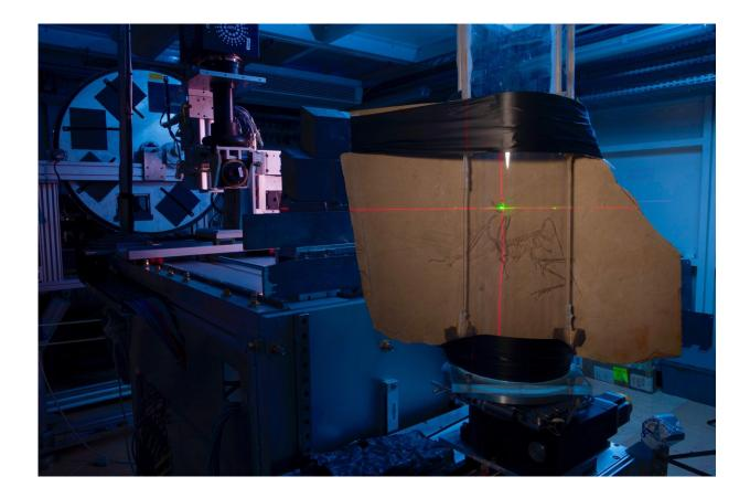
The Munich specimen of *Archaeopteryx* at beamline ID19 at the ESRF. The limestone plate was mounted on a rotating sample stage and the beam is here centered on the skull using lasers. The X-ray beam, coming from the right of the picture, travels through the sample and arrives at the detector (visible left) where a camera records the signal. Credit: ESRF/Pascal Goetgheluck
