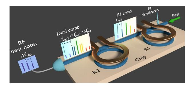
A compact, integrated, silicon-based chip used to generate dual combs for extremely fast molecular spectroscopy. Credit: A. Dutt, A. Mohanty, E. Shim, G. Patwardhan/Columbia Engineering
