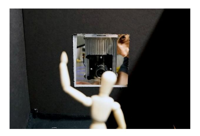
The MIT system was able to resolve images of objects and gauge their depth at a range of 57 centimeters. Credit: Melanie Gonick/MIT
