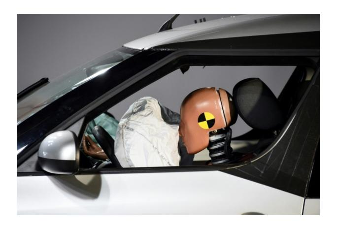
Airbags contain a chemical propellant which can inflate a bag within 0.0005 seconds
