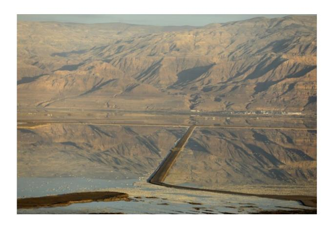
Evaporation ponds at the southern part of the Dead Sea where both sodium chloride and potassium salts are produced
