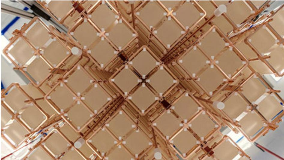
Bottom view of the 19 CUORE towers installed in the cryostat. Credit: Yury Suvorov, University of California and INFN Gran Sasso National Laboratories, and the CUORE Collaboration
