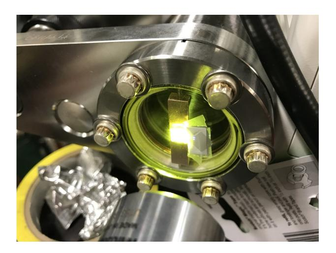
X-rays strike a scintillator material at the COSMIC beamline, causing it to glow. Credit: Simon Morton/Berkeley Lab
