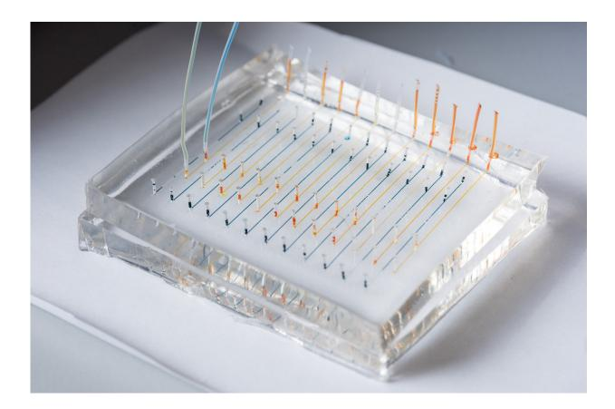
This close-up image shows a microfluidic chip used to fabricate nanoparticles that could be used to deliver therapeutic genes to specific organs of the body. Colored liquids have been added to highlight the channels. Credit: Rob Felt,
