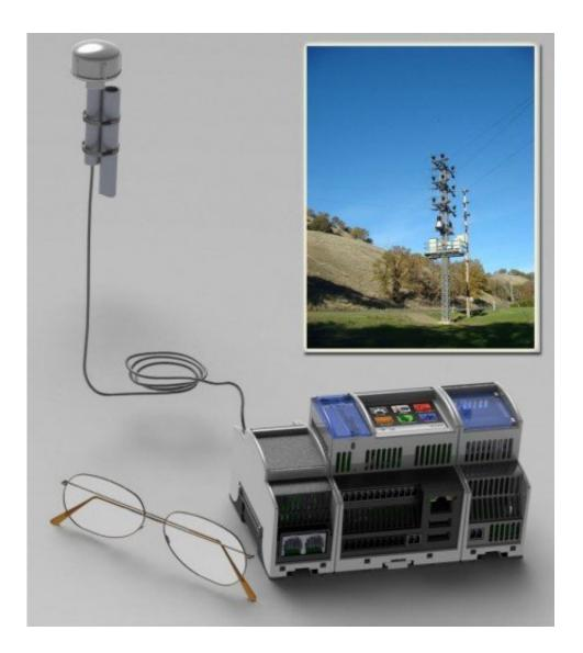
Developed at Power Standards Lab under a project led by UC Berkeley and funded by the Department of Energy's ARPA-E program, µPMUs are designed to increase situational awareness at the power distribution grid level. Credit: Power Standards Lab
