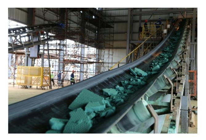
Chunks of cobalt that have undergone preliminary processing at a plant in Lubumbashi. The ore is then exported, mainly to China, to be refined
