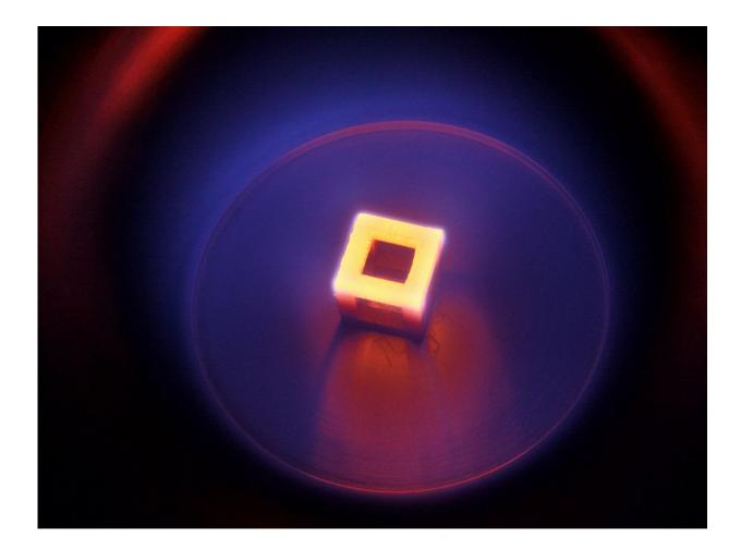
3-D printed titanium in a CVD plasma chamber. Samples glow due to the heat of the microwave plasma, once removed the titanium will have been coated with diamond. Credit: RMIT University
