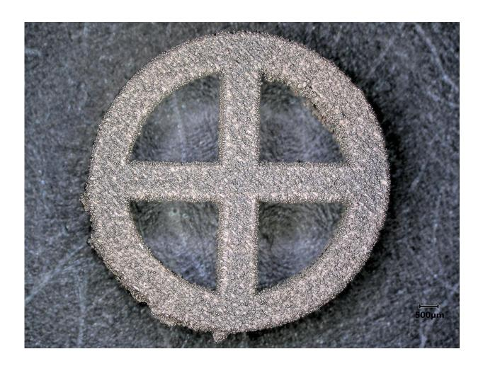
A diamond coated 3-D printed titanium disc. Credit: RMIT University
