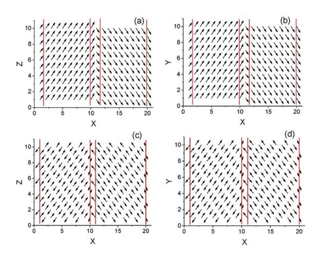
The red lines in these images illustrate the domain walls separating regions of electric polarization (top) and shifting of charged ions (bottom row) in a material called bismuth ferrite. Researchers have demonstrated that these domain walls can be used to transmit a type of electrical current, which could lead to novel electrical devices. Credit: Sergey Prosandeev
