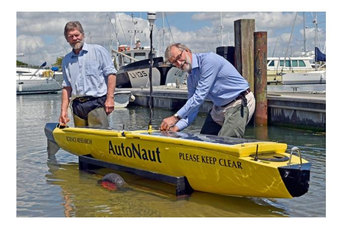
A new company from ESA Business Incubation Centre Harwell in UK has developed the autonomous AutoNaut boat that is propelled by the waves and carries ocean sensors powered by solar energy. Credit: European Space Agency
