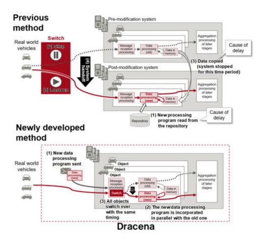
Figure 2: Differences between the existing technology and Dracena's non-disruptive update technology. Credit: Fujitsu
