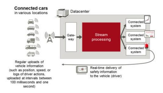
Figure 1: Real-time services via the collection, analysis, and utilization of data from connected cars. Credit: Fujitsu
