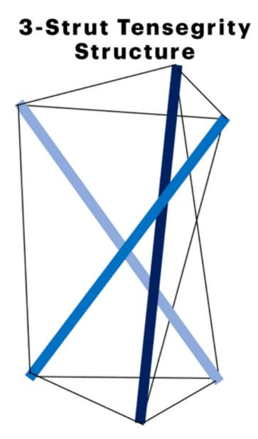
One of the simplest tensegrity structures – three stiff rods (blue) held up into a
