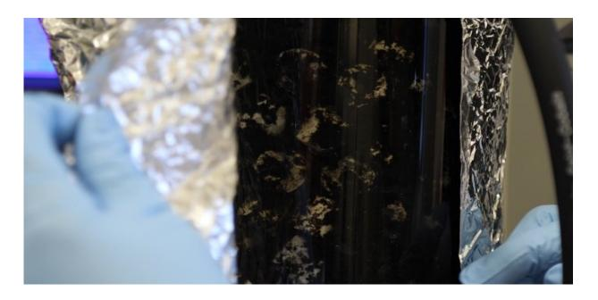
Anaerobic bacteria attach themselves on packing media placed inside the anaerobic bioreactor. Credit: King Abdullah University of Science and Technology
