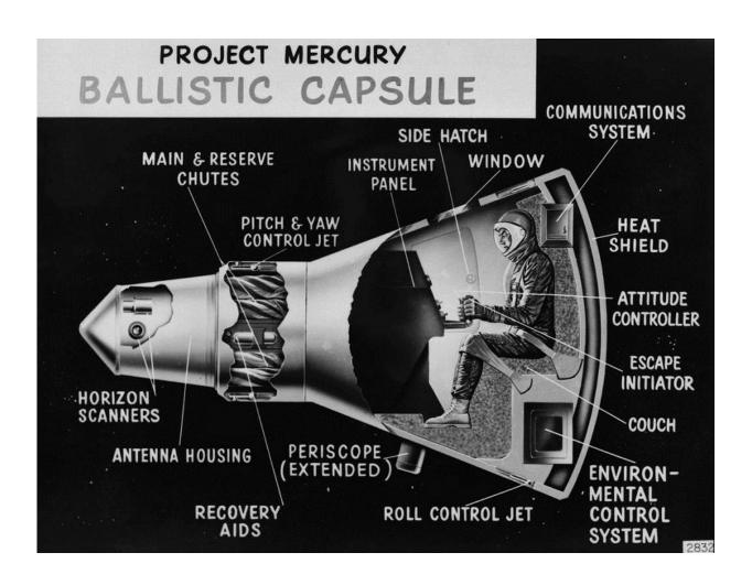
Less than a year after its birth, NASA announced Project Mercury, the first American attempt to send a person to space. Project Mercury proved that humans could live and work in space, paving the way for all future human exploration. This cutaway drawing of the Mercury capsule was used by the Space Task Group at the first NASA inspection, on Oct. 24, 1959. Credit: Courtesy of NASA.
