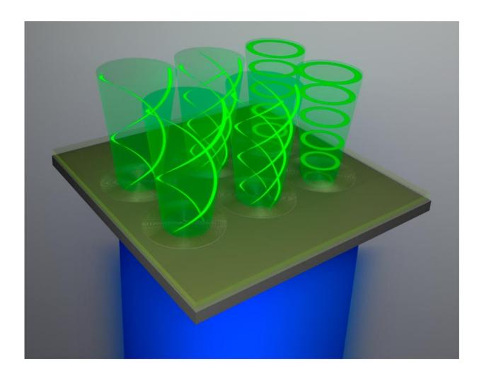
Illustration of an array of organic vortex lasers, each with a different spiral and therefore a different topological charge. Credit: Stellinga et al. ©2018 American Chemical Society
