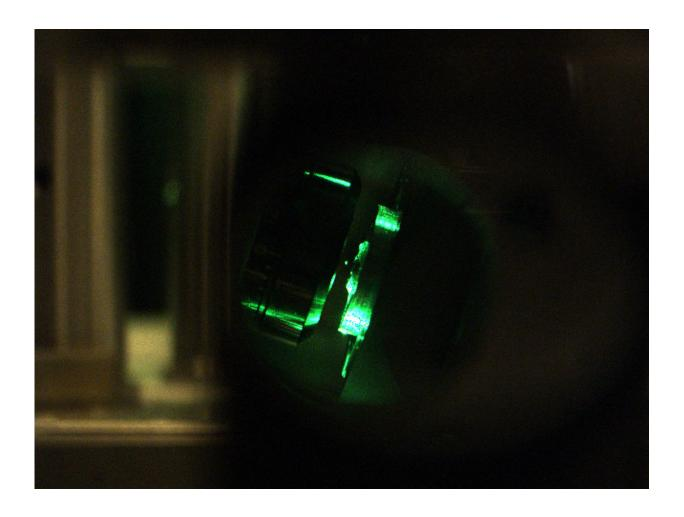
Researchers experimentally tested the differential fluctuation theorem using an optically levitated nanosphere which can be trapped in air continuously for 65 weeks, acquiring large sets of data. Credit: Tongcang Li
