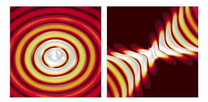
Illustration of waves propagating away from a point-like source. Left: Regular wave propagation. Right: Wave propagation on a hyperbolic metasurface. Credit: P. Li, CIC nanoGUNE
